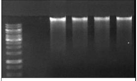
Agarose Gel analyzed by electrophoresis Bacterial DNA isolated from GeneFiX Saliva Microbiome DNA collector using Saliva-Prep-2 shows quality DNA with no degradation
