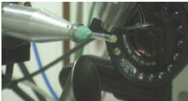
Figure 12: Single channel cut from CrystalSlide™ and mounted in front of an X-ray beam (APS GM/CA CAT ID-D) for in situ X-ray screening.
