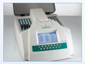
The ESR tubes 1.5ml are used for Erythrocyte Sedimentation Rate measurement on the Greiner SRS and SRT instruments.
