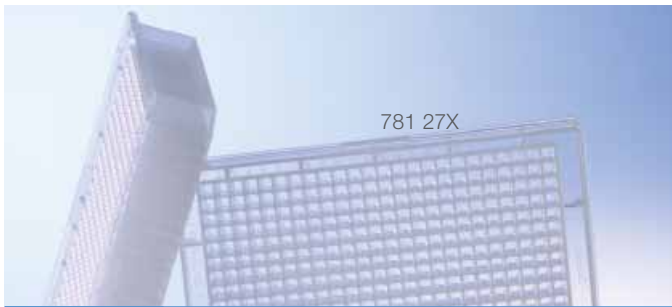
Figure 1: Well profile: 384 Deep Well MASTERBLOCK®, polypropylene Total volume: 240 µl Working volume: 20 – 225 µl
