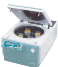
Please note that incorrectly prepared centrifuges deliver poor quality samples. A normal use laboratory centrifuge (with a radius of approximately 180mm) corresponds to: 150g approx. 900 revolutions per minute, 1500-2000g approx. 3000 revolutions per minute and 2500-3000g approx. 4000 revolutions per minute.
