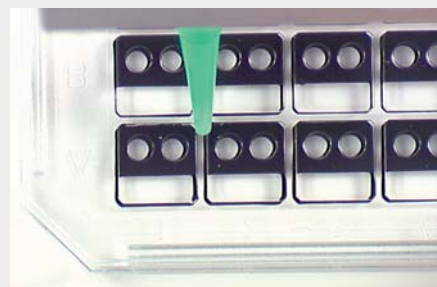
Figure 7: Pre-greasing of CrystalDrop™ lid
