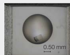
Figure 5 b): Crystallisation of lysozyme in CrystalQuick™ LP, RoboDesign International Inc., Carlsbad (USA)
