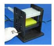
This manifold can also be sterilized by autoclave and used to aspirate sterile media.
