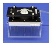
The BMPJANUS-SM mounting plate is adjustable in the Z direction with 4 individual thumbscrews that can be locked in position. This feature allows the operator to adjust the aspiration tubes to be same distance to microarray slide. A bubble level is included is included to assist in this adjustment.
