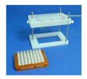
The height of the manifold is easily adjusted by loosening the thumb screws and sliding the manifold up or down on the stainless steel rods as shown in the photo on the right.
