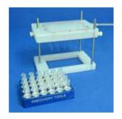
The height of the manifold is easily adjusted by loosening the thumb screws and sliding the manifold up or down on the stainless steel rods as shown in the photo on the right.
