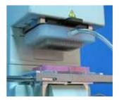
The photo to the right demonstrates the 384 aspiration manifold mounted to our very own V&P Pin Tool Robot using a BMPAPRICOT mount.
