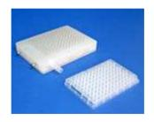
These manifolds are resistant to acids, bases and organic solvents as they are made with a rugged polypropylene body and 13 mm long 20 gauge stainless steel tubes. The shoulder bolts register the manifold to the Jig and the Jig can be adjusted in all 3 axis (X, Y, and Z) for perfect positioning of the tubes between the wells. The alignment of the plates with the tubes is a snap.
