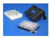
96 Slant Tube Aspiration Manifold, vertical tube length 12.6 mm, OD = 1.06 mm, ID = 0.66 mm, 19 gauge, guide pins cut so tubes are 1 mm above well bottom  $^{\circ}$
