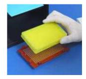
The VP 771G-4 uses very strong 48 Megagauss Oersted NdFeB Magnets to facilitate rapid capture of the magnetic beads.
