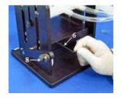
The photo on the right illustrates (7) the Z height adjustment knob. The Z height can also be adjusted by how far down in the slots the Manifold shoulder bolts (2) are positioned. These two Z positioning mechanisms provides great flexibility so both standard and deep well microplates can be accommodated by the same Jig.
