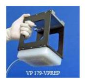
The Agilent (Velocity 11) V-PREP mounting Fixture was attached to a customized 384 well aspiration manifold (VP 179-BJ) via a custom standoff (black) that accommodates for the height of V-PREP pipetting head and has a rotation adjustable plate.
