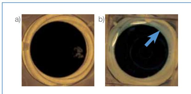
**Figure 4:** Wells filled with methylene blue after threefold freezing and thawing: a) single well of a Greiner Bio-One UV-Star® microplate b) single well of a 96 well UV-transparent microplate of a competitor
