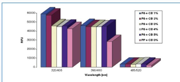
**Figure 6:** Influence of the black pigment fraction and the wavelength used on the autofluorescence of 96 well microplates
