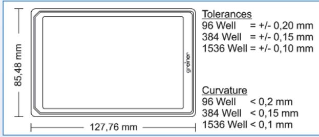
Figure 1: Footprint and tolerances of standard microplates
