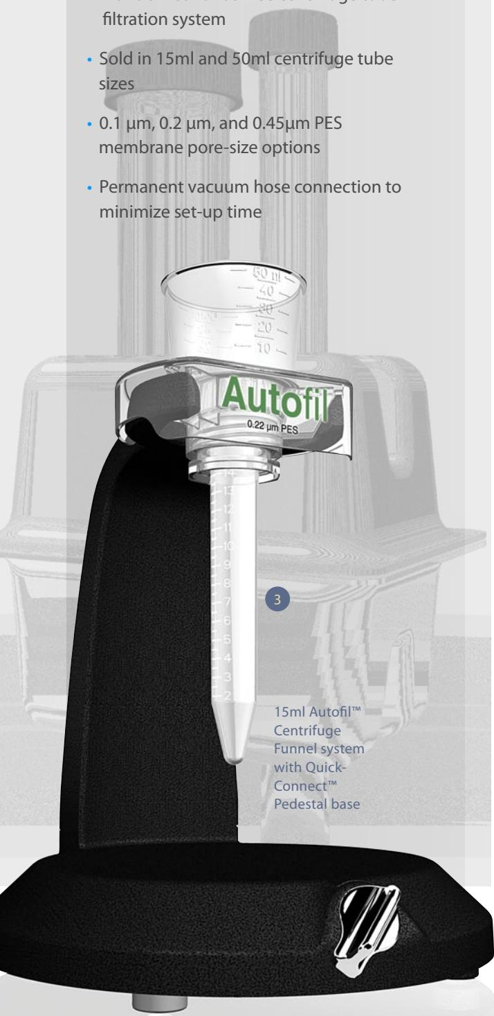
Foxx Life Sciences has developed the world's first hands-free centrifuge tube filtration system. Each filtration unit includes a sterile centrifuge tube and cap, 50ml funnel with PES membrane, funnel adapter (for the 15ml tube assembly), vacuum hose adapter, and dual centrifuge tube stand.
